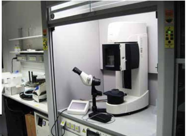
Fig. 2: Automatic plunge freezer.
