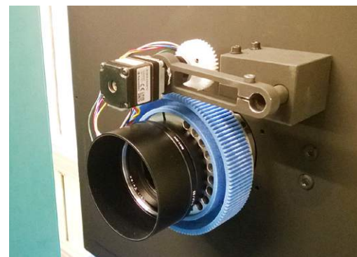
The remote controlled focussing unit with dismounted bellow.
