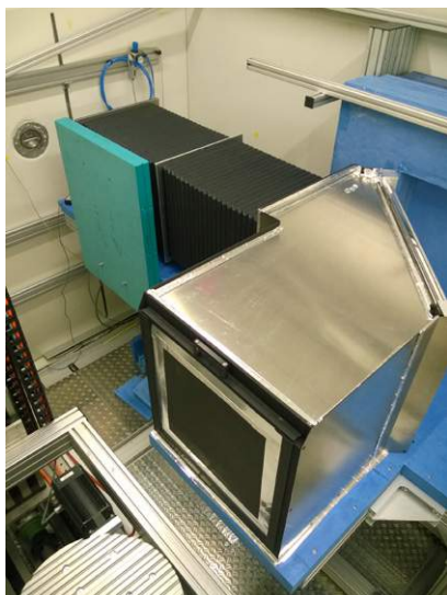
The new detection system during commissioning phase. In the foreground is the turntable of the sample manipulator. In the upper left part the two bellows are visible, one partly hidden by a vertically fixed (green) borated PE plate used for the investigation of the influence of scattered radiation by samples. The aluminum tapes for testing the light-tightness of the housing will be removed.
