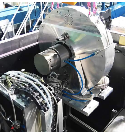
Fig. 3: Installation of the TISANE chopper disk at SANS-1 (Nov. 2015).
