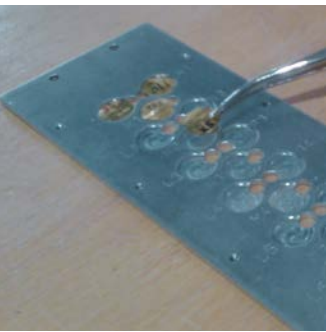
Placing the gold foils into the holder with a cross section of 3 \times 17 cm.
