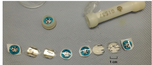
Fig. 1: Thermometer labels and standards after irradiation in the rabbit system.
