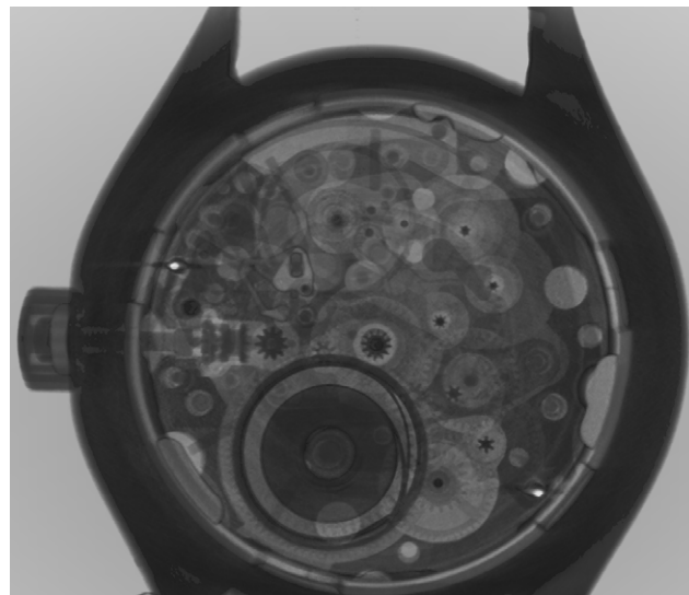
Fig. 1: A reconstructed neutron tomography of a mechanical watch acquired with a prototype high resolution boron-based neutron scintillator screen.
