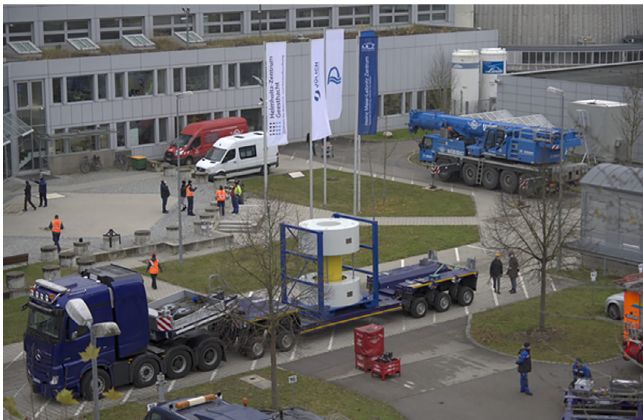
Fig. 1: It takes a lot of equipment to handle the CASTOR® MTR 3 cask. The cask in the picture is only a dummy used for training purposes.
