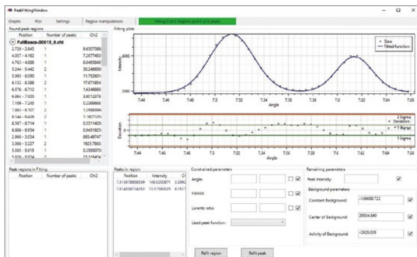
Figure 1: Screenshot of the peak-fitting window of DISEMM, including plot of the fit, plot of deviation between calculated and measured intensities, peak list and values of selected refineable parameters.
