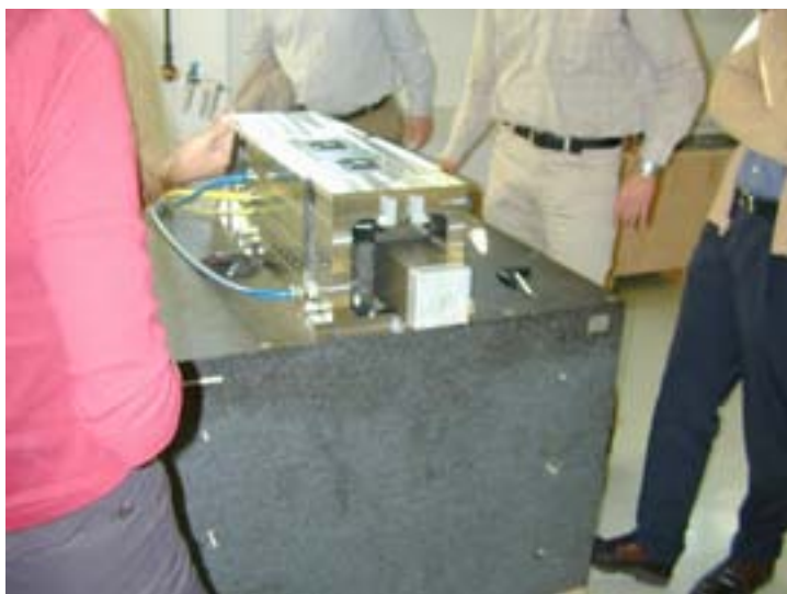
Figure 3.15: Test run of the final version of the Doppler drive at 4.7 m/s
