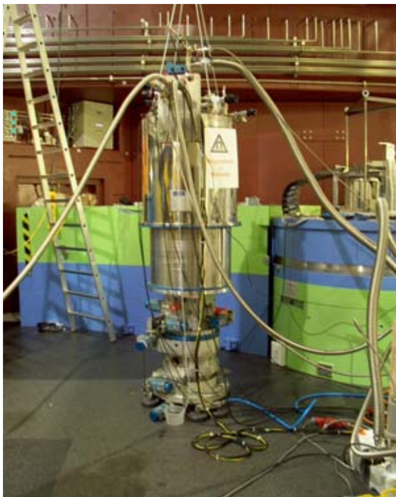
Figure 3.8: 15T vertical magnet on the PANDA sample table
