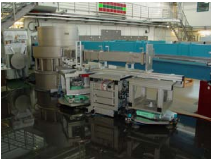
Figure 3.1: The reflectometer option of MIRA without the detector and the magnets for the guide field.
