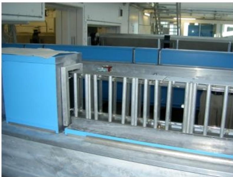
Figure 3.12: magnetic guide field for the polarising guide
