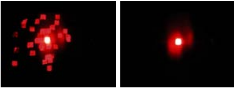
Figure 3.16: A quality check of the high-resolution analyser. Left the very first test waver that was glued, to the right a good average image.
