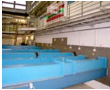
Figure 1.9: The accomplished wall of the NG hall. On the final steel cover several shock sensors of the safety system are visible. All NG are jacketed by the (blue) lead plates.
