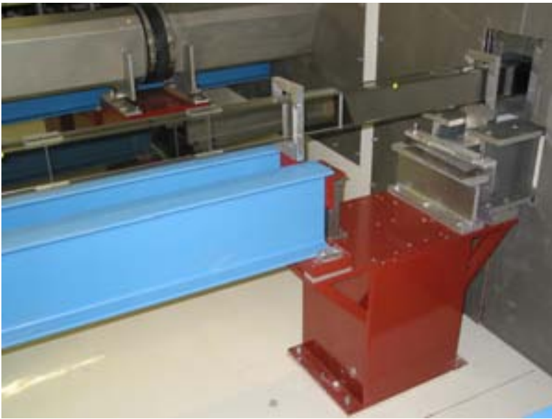
Figure 4.6: Section of the guide NL3a which will transport cold neutrons to MEPHISTO. The support socket shown is situated six meters upstream from the end of the guide. The glass elements can be easily reconfigured to accommodate a neutron polariser and choppers or a velocity selector on the socket.
