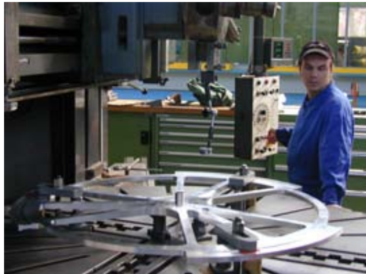
Figure 3.14: The intermediate version of the chopper wheel during centering of the central bushing
