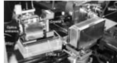
Figure 7.8: X-ray optics of the Bragg Magnifier. Both crystals in Kirkpatrick-Baez geometry as well as the entrance of the 1:1 tandem optics are clearly visible.
