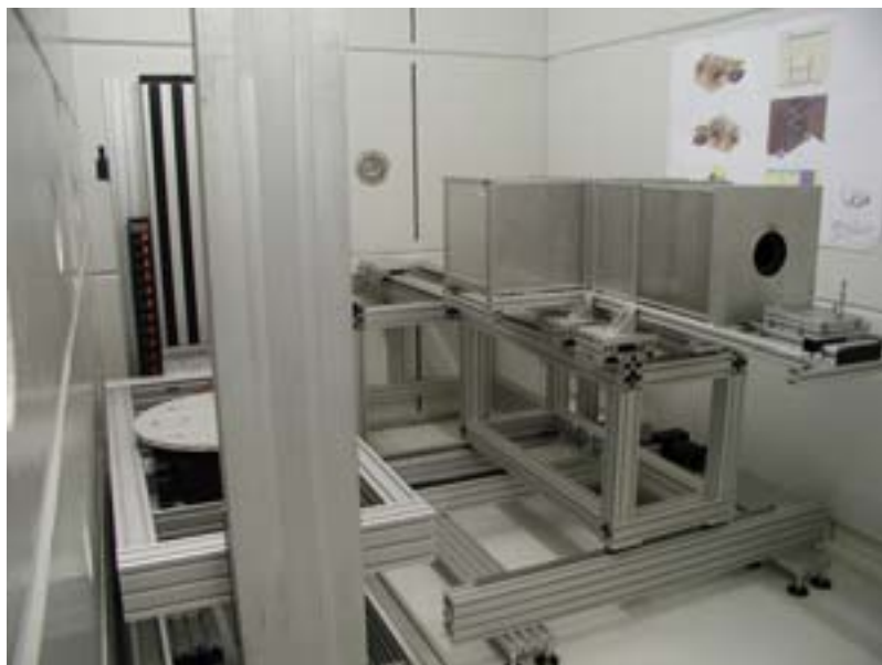
Figure 5.6: View in the measuring room with manipulator system for the objects (left), for the detectors (right) and provisionally mounted two-dimensional detector system (without CCD-camera).
