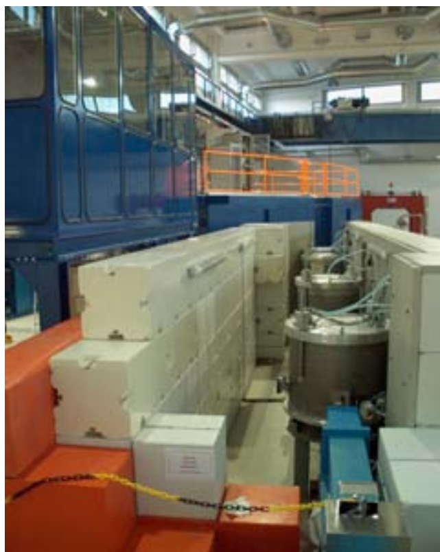
Figure 3.18: Front view of the time-of-flight spectrometer at FRM-II with disassembled shielding of the primary spectrometer (see text)
