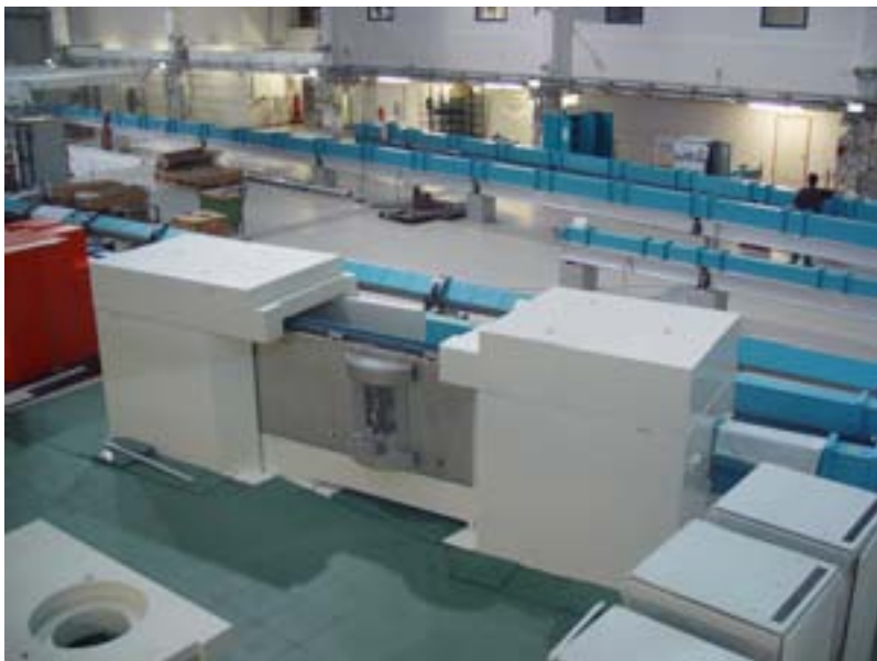
Figure 2.6: Monochromator shielding at the cold neutron guide NL-1 in the FRM-II guide hall with sliding front wall (including the rotating drum) in place.
