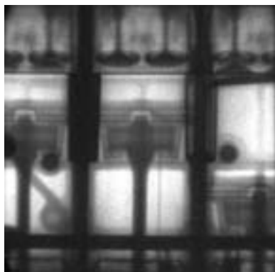
Figure 6.13: Piston cooling of a four stroke car combustion engine can be observed well by neutron radiography, t=200 ms with 120 accumulations, image size is 24cm x 24cm
