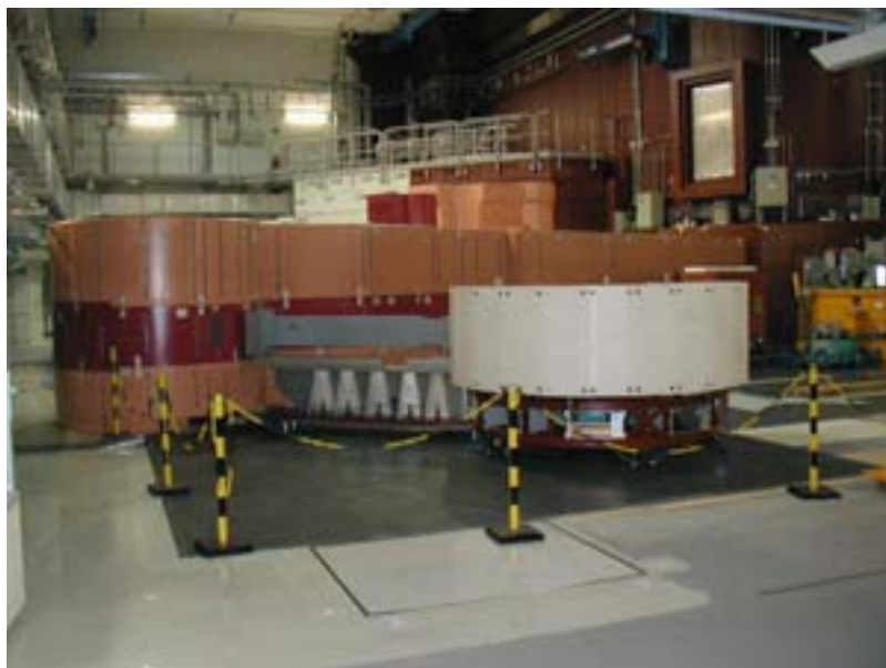
Figure 2.15: Side-view on instrument SPODI with shielding of the neutron guide & monochromator and detector in the foreground
