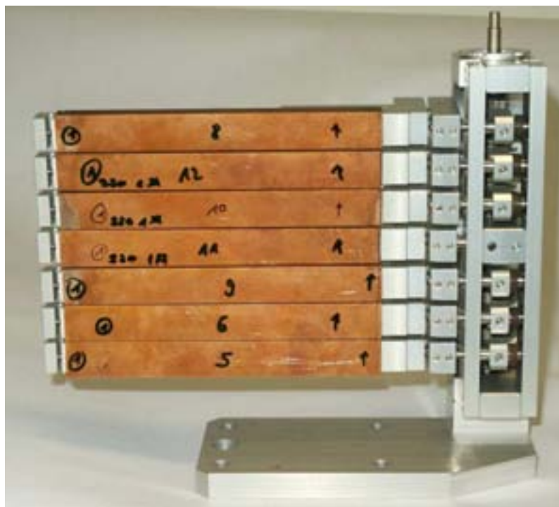
Figure 2.5: Focussing unit with mounted Cu-(220) crystal
