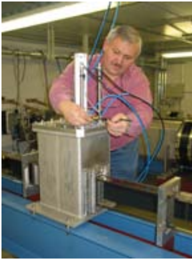
Figure 4.8: J. Fink mounting the shutter in the NL3a beamline.
