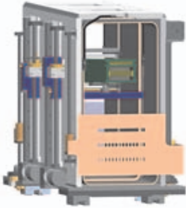
Figure 2.10: Neutron optical body in the beam guide chamber with the mechanics for vertically aligning a NGE and an ancillary diaphragm.
