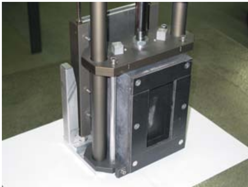
Figure 4.7: The secondary beam shutter (technical design: F. Tralmer). Its vacuum housing also includes two movable beam attenuators, visible behind the shutter block.
