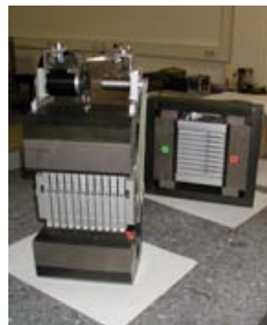
Figure 3.7: The focussing mechanics for the Heusler crystal analyser (foreground) and monochromator (background)
