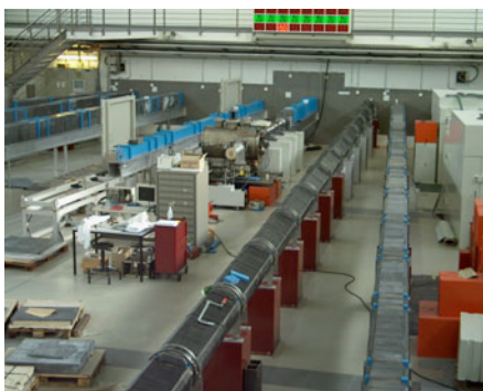
Figure 1.6: View of the NG NL 2a and NL 2b in the NG hall. The NG NL 2b (left) is in the state of being wrapped with boron foam sheets. The NG NL 2a (right) is being equipped with additional lead plates.
