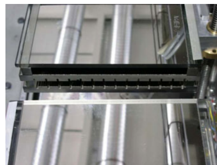
Figure 2.13: View of neutron guide element 3 with its upper channel used for continuing NL-2b (height: 12 mm; width: 170 mm) and its lower channel designed as a radial pre-collimator.
