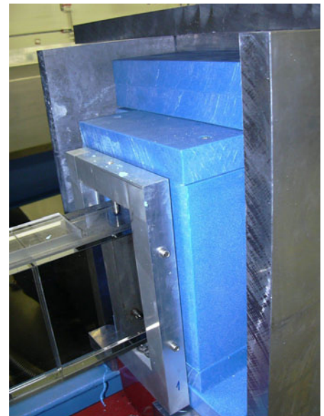
Figure 1.7: Looking at the shielding structure of the NG in the casemate during the assembling period. The glass body of the NG is enclosed by two layers of boron treated PE (blue). They are covered with lead plates (grey).
