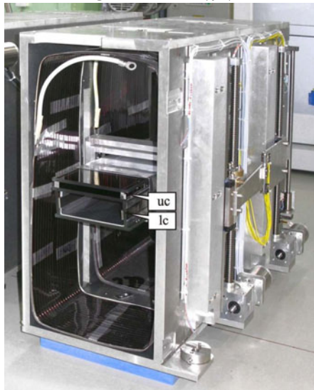
Figure 2.14: View of a neutron optical body of the beam guide chamber with the mechanics for vertically aligning a NGE. The NGE consists of an upper channel (uc) for continuing NL-2b (height: 12 mm; width: 170 mm) and a lower channel (lc) designed for vertically collimating and keeping the large horizontal beam divergence.
