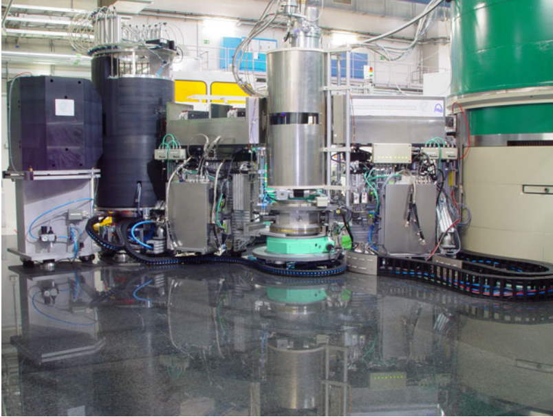
Figure 3.11: The TRISP spectrometer [1] at the FRM-II is operational. In a first study, of magnon linewidths in the antiferromagnet \text{MnF}_2 , an energy resolution as low as 1\mu\text{eV} was obtained. The polarized neutron flux of 4 \times 10^7 \text{cm}^{-2}\text{s}^{-1} at the sample (at k_i = 3\text{\AA}^{-1} ) is competitive with the best polarized TAS instruments [2]. The background is very low (1 count per 10 min).
