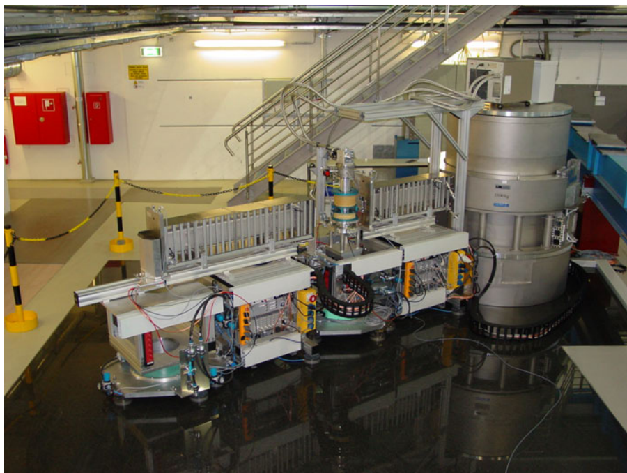
Figure 2.5: MIRA in the polarised reflectometer option equipped with a magnet and a closed cycle cooling machine.
