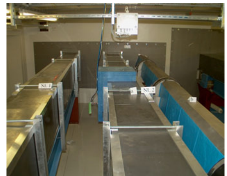
Figure 1.8: View of the NG NL 1, NL 2a and NL 2b in the casemate after accomplishment of the rather massive sandwich shielding.
