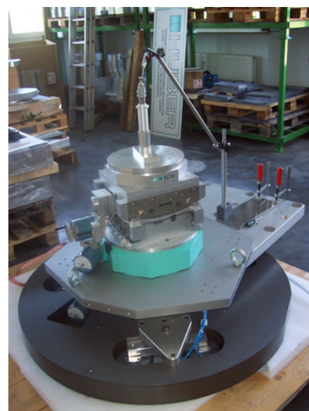
Figure 2.11: Non-magnetic sample table for the new diffractometer POLI-HEiDi during the acceptance tests.
