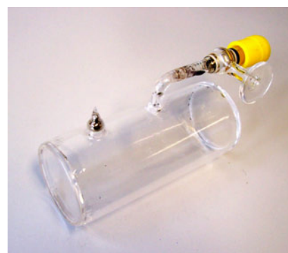
Figure 2.8: Spin filter cell Heidi 4.1 made of quartz glass and Cs coated inside. J. Young type greaseless high vacuum stopcock is used in the edge geometry.
