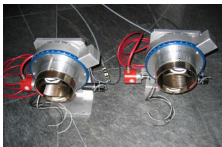
Figure 2.12: Adiabatical spin rotators from the axial to the transversal direction regarding the beam propagation direction (nutators) fixed on their mechanical turn tables.
