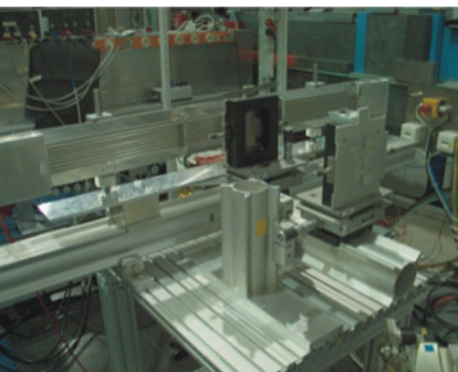
Figure 1.1: Prototype detector consisting of 8 PSDs mounted at TREFF during the PSD8+ readout system test
