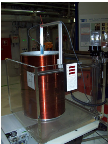
Figure 2.9: Main coil of the Decpol during the magnetic field test measurements.
