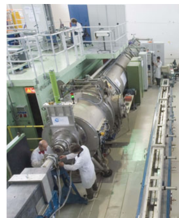
Figure 2.15: View of the KWS-2 SANS instrument at FRM II (summer 2007); on the right side the open collimation housing of KWS-1 SANS instrument can be seen.
