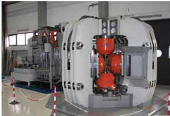
Figure 12: The multi-anvil press of the instrument SAPHIR in the Neutron Guide Hall East.
