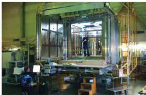
Figure 10: The passive shield with a very small magnetic field inside.
