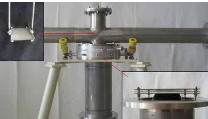
Figure 1: The experimental setup. The Uranium target (upper left) is placed in the horizontal beam line. The beta spectrum is recorded by a module consisting of a multiwire chamber and a plastic scintillator (lower right).
