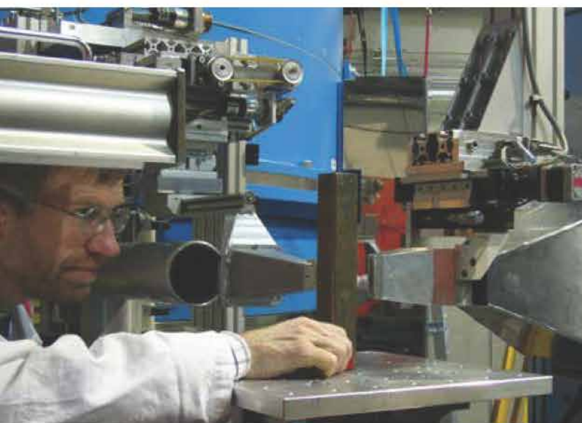
Figure 1: Alignment of a sodium-iron chloride battery cell on the sample table of STRESS-SPEC.
