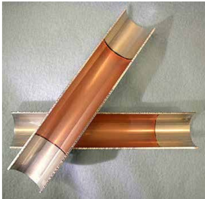
Figure 2. Inside of a copper-coated target cylinder.
