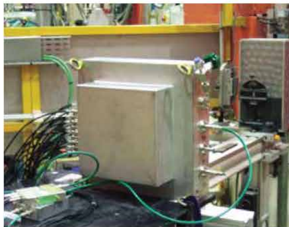
Figure 2: The GSPC19 detector mounted at CT2 beam line at ILL for a first integration test.
