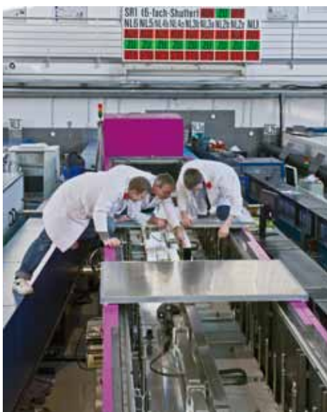
Fig. 2: Gerd Musielak, Juri Stell and Oliver Frank of HZG insert the apertures in the collimation system.
