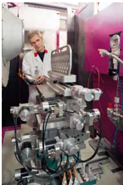
Fig. 3: Ralph Gilles (TUM) testing the sample tower with the manual control.
