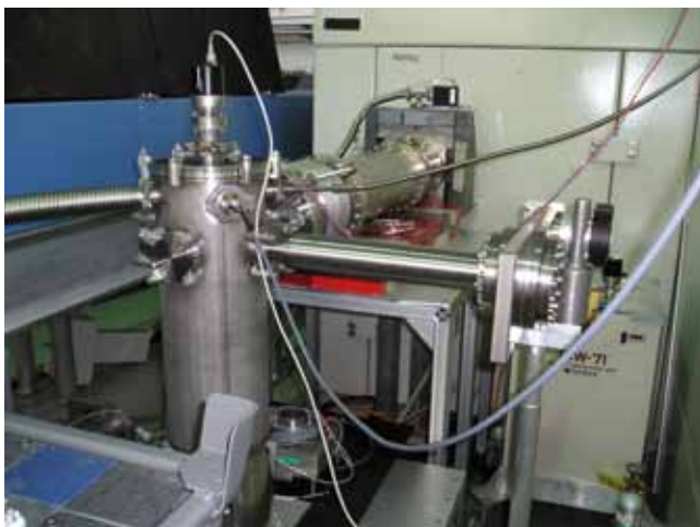
Fig. 4: UCN cryo converter partly dismantled.
