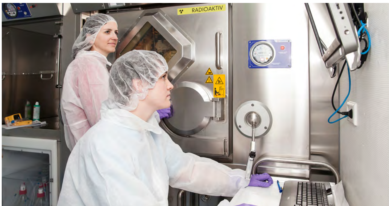
Figure 1: Grade A environment for the production of n.c.a. Lu-177.
