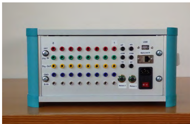
Figure 4: Plug'n Play digital I/O box to be used easily with TACO and NICOS instrument control software.
