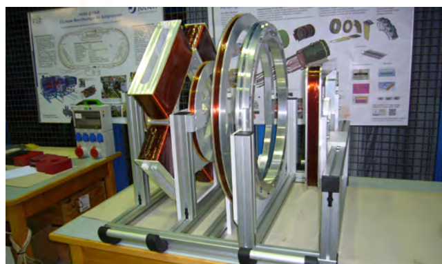
Figure 21: (Top) Schematic of the coil and magnet layout for the preparation and analysis of the neutron polarization. (Bottom) Image of the coil and magnet configuration for the preparation of the initial neutron polarization on the frame for the 3-d mapping of the field distribution.
