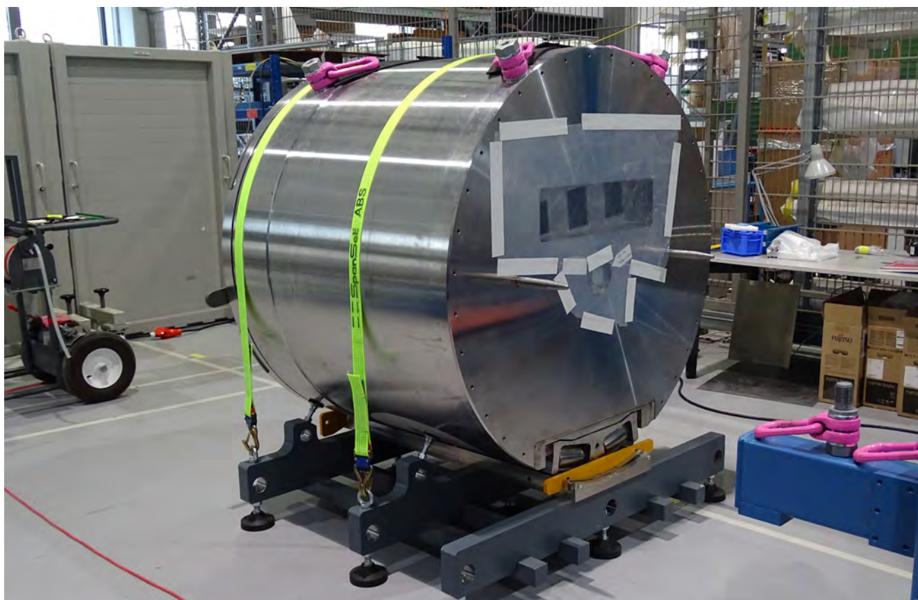
Figure 2: New plug for beam tube SR5, a highly engineered heavy weight of steel, concrete and advanced shielding.
