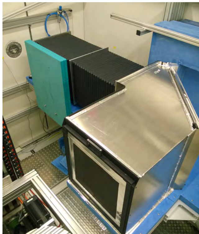
Figure 4: Picture of the new NECTAR detector system. The turn table of the sample manipulator is visible on the lower left in front of the new scintillator (lower center) and the fixed aluminum part of the detector box. The backing of the foil mirror can be seen on the right-hand side of the picture at the "elbow" of the box. On the upper left the new bellows surrounding the movable part of the box can be seen shielded against scattered radiation from the samples by a vertically fixed borated PE plate.
