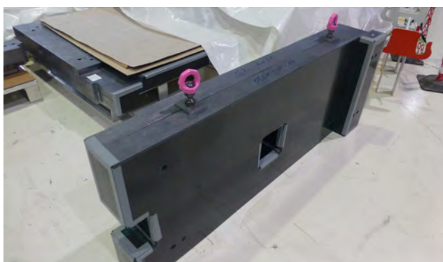
Figure 23: Assembly of the radiation shields for KOMPASS.
