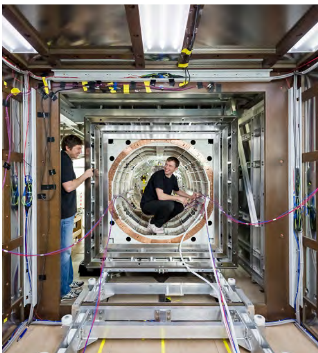
Figure 3: The weakest magnetic field in the solar system was one of the striking items of news this year and this record-breaking magnetic shielding for high-precision experiments stands in the new guide hall east at the FRM II.
