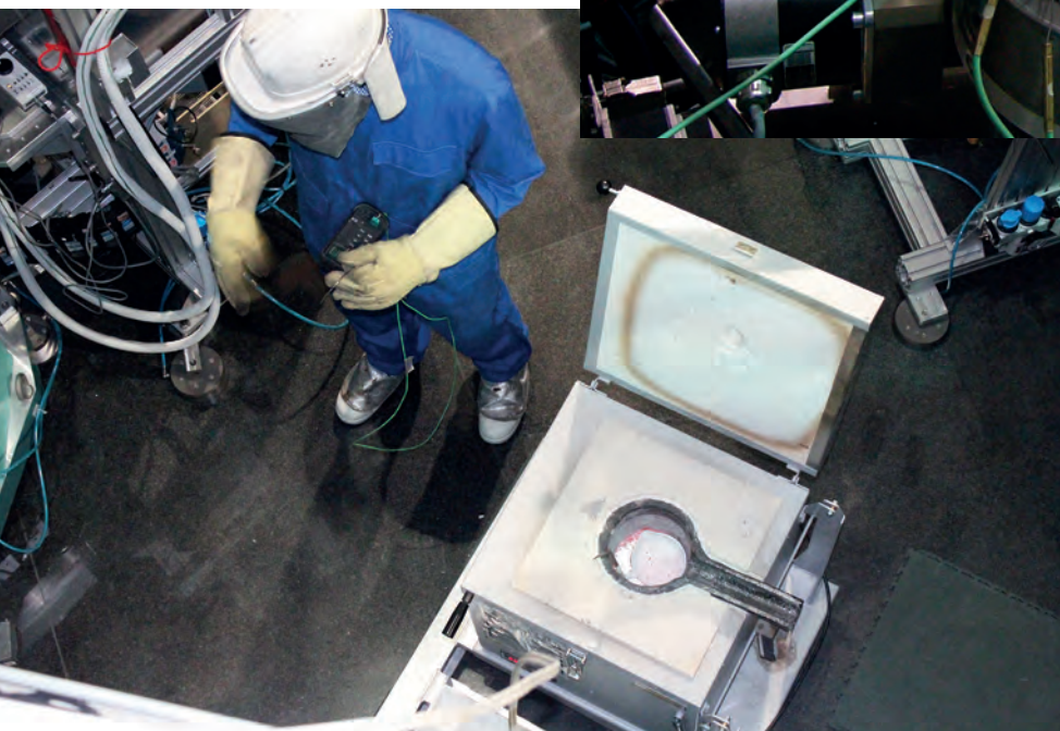
Fig. 2: The next step was heating Al in a melting furnace to casting temperatures of about 700°C.
