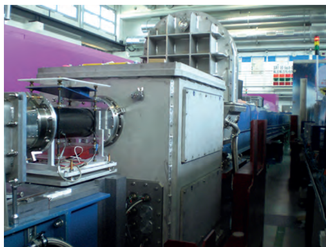
Fig. 4: Chopper chamber, polarizer chamber and spin flipper (the big installation in front of the collimation).
